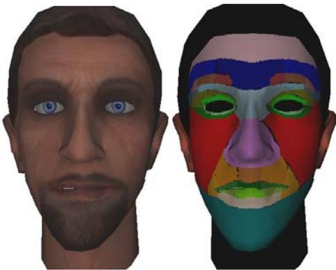
**Figure 5. Face Regions. These are small areas that usually move together and are controlled by Feature Points. iFACE Components are related groups of these Regions, e.g. eye area**
